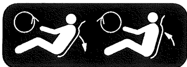
Adjustment winch of the backrest
