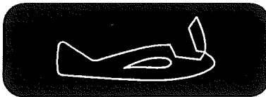
White levers for opening the canopy
